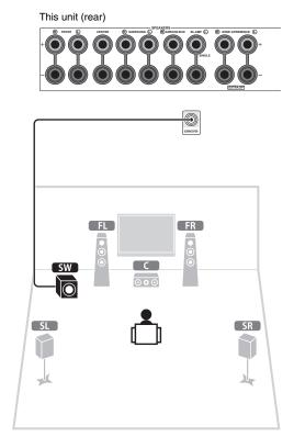
Use an audio pin cable to connect the subwoofer (SW).
