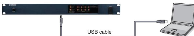
Do not connect the devices in a network until the IP addresses have been set. To set the IP addresses, connect PC to each device in turn, using a USB cable.
