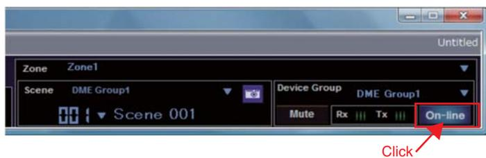
When the Synchronization window is displayed, the text "Select IP Address" will be displayed in red. Click this message and select the required IP address from the drop-down menu.
