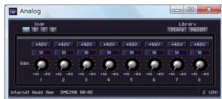
By default, the gain is set to +10 dBu (i.e., the lowest possible level). Adjust the sensitivity to the correct level for the connected audio equipment.
