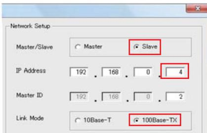
Select [100Base-TX] in the Link Mode area of the Network Setup window for both the DME8o-C and the DME64N.
