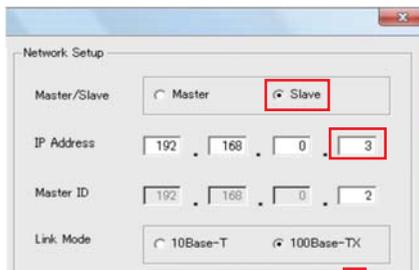
Select [Slave] in the Master/Slave area of the Network Setup window for both the DME8o-C and the DME64N.
