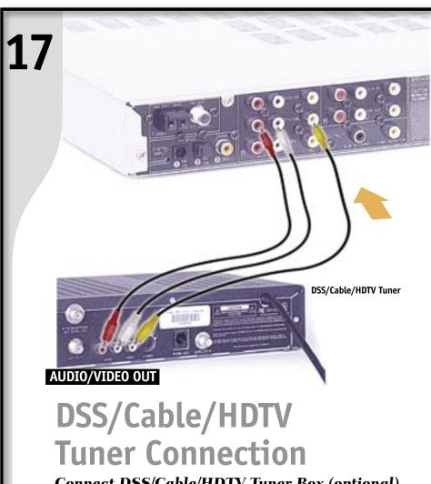
**Connect DSS/Cable/HDTV Tuner Box (optional)** Connect RCA audio/video cables (not included) or optical cable (not included) to "DTV/CBL" terminals on receiver as shown.
