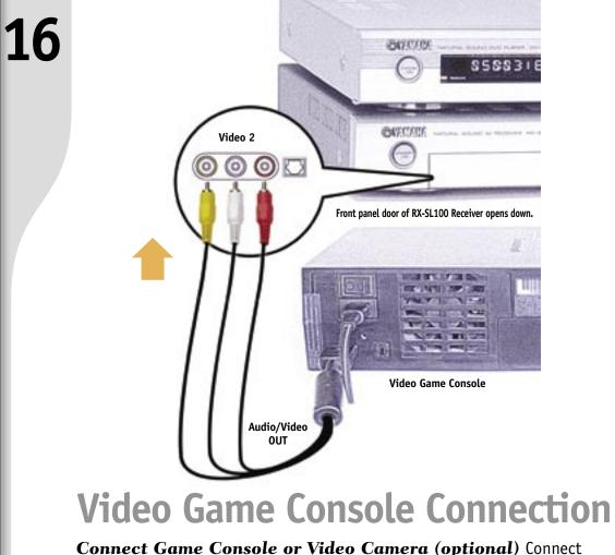
Connect Game Console or Video Camera (optional) Connect RCA audio/video cables (not included) or optical cable (not included) as shown.
