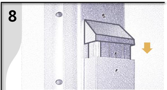
**Attach Finishing Brackets 7** on top of two speaker stands.
