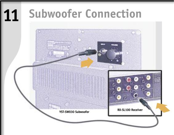
**Connect RCA Cable** Unplug subwoofer **12** before proceeding. Connect RCA cable 8 to subwoofer. Set subwoofer VOLUME control to half-way mark and POWER to OFF. Connect RCA cable to receiver from subwoofer.
