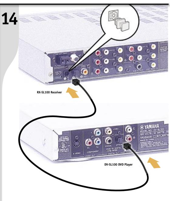
**DVD Player Optical Connection (optional)** Remove dust cap on optical input as shown on inset. Connect optical cable (not included) to receiver. Connect optical cable to DVD player from receiver.
