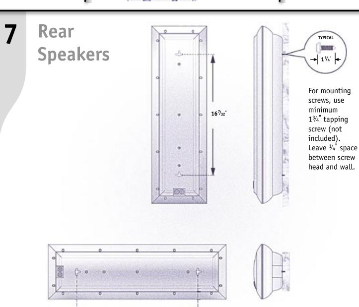
**Mount Surround Speakers and Surround Back Speaker** Fasten mounting screws into a firm wall or wall support as shown. Hang the keyholes on the back of the each of the speakers ② on the protruding screws. Attach speaker wire as shown in Step 6.
