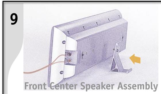
**Attach Bracket and Speaker Wire** Attach bracket **11** to center speaker **3** using supplied screw as shown. Attach speaker wire as shown in Step 6.
