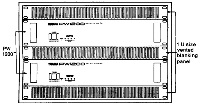
Rack mounting with vented blanking panels
