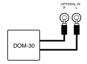
These jacks are intended for use with an external tone generator module such as the Yamaha DOM-30 Disk Orchestra Module. The stereo outputs from the external tone generator module are connected to the OPTIONAL IN L and R jacks, allowing the sound of the tone generator to be reproduced via the Clavinova's internal sound system and speakers.
