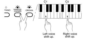
Depending on which voices you combine using the DUAL mode, the combination may sound better if one of the voices is shifted up an octave. To shift the right voice, press the C5 key while pressing the two voice selectors corresponding to the voices to be combined in the DUAL mode. Press C5 again to shift the voice back to its normal range. Use the C1 key in the same way to shift the left voice.
