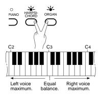
The volume levels of the two voices combined in the DUAL mode are normally set automatically to produce a pleasing balance (see "Default Settings" below). The balance can be adjusted manually by using the C2 through C4 keys on the keyboard while pressing the two voice selectors corresponding to the voices to be combined in the DUAL mode.
