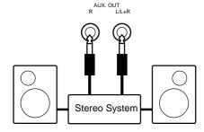
The AUX OUT R and L/L+R jacks deliver the output of the Clavinova for connection to an instrument amplifier, mixing console, PA system, or recording equipment. If you will be connecting the Clavinova to a monaural sound system, use only the L/L+R jack. When a plug is inserted into the L/L+R jack only, the left-and right-channel signals are combined and delivered via the L/L+R jack so you don't lose any of the Clavinova's sound.
