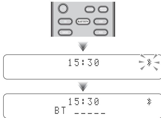
Press the **BLUETOOTH** source button to switch the audio source to *Bluetooth*.
