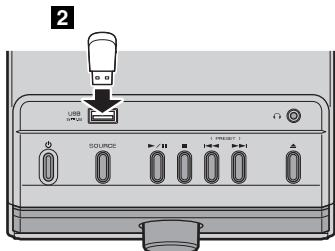
**1** Press the **USB** source button to switch the audio source to USB.
