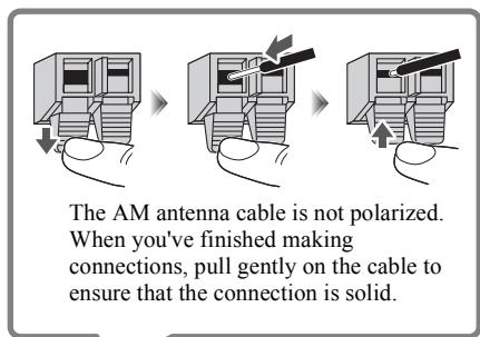
The AM antenna cable is not polarized. When you've finished making connections, pull gently on the cable to ensure that the connection is solid.
