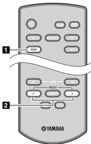
**1** Press the **RADIO** source button to switch the audio source to FM or AM.
