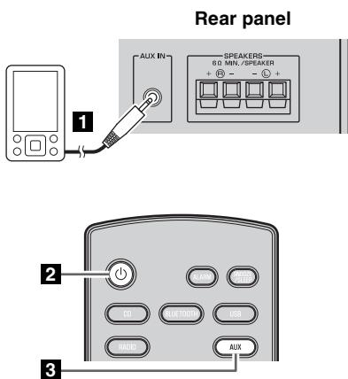
**1** Using a commercially available 3.5 mm stereo mini-plug cable, connect your external device to the **AUX** jack on the rear panel of this unit.
