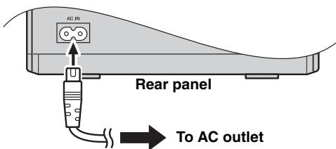
When you've completed all connections, connect the supplied power cable to AC IN, and then connect the plug of the cable to an AC outlet.
