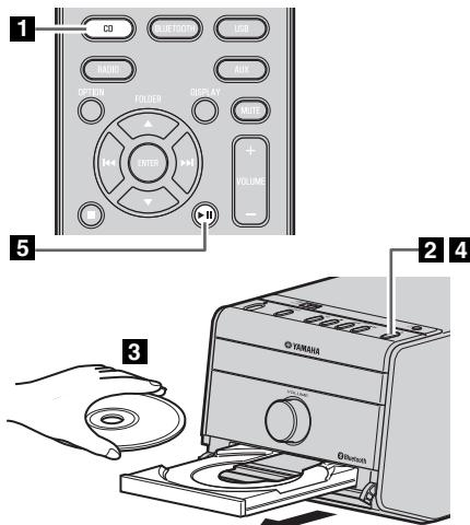
**1** Press the **CD** source button to switch the audio source to CD.
