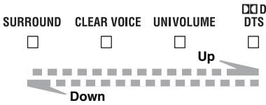
The color of **DTS** indicator changes depending on the adjustable range. Green indicates a lower volume level, orange a moderate level, and red a higher level.
