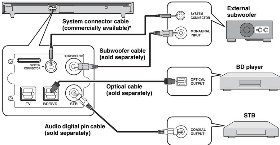
\* If connecting an external Yamaha subwoofer, use the cable supplied with the subwoofer to enable synchronous on/off switching of the unit and subwoofer.
