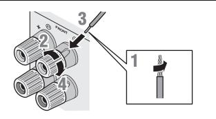
Remove approximately 10 mm of insulation from the ends of the speaker cables, and twist the bare wires of the cables together firmly so that they will not cause short circuits.
