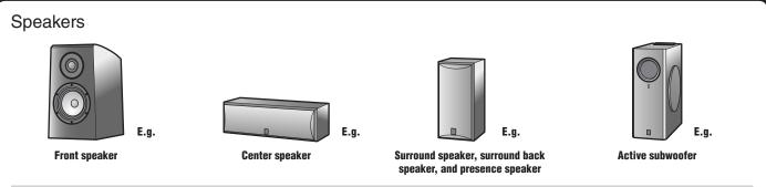
Use speakers with an impedance of at least 6Ω. 4Ω speakers can also be used as the front speakers. For more information on speaker impedance, refer to page 3.
