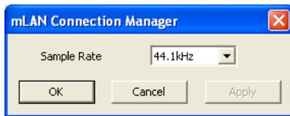
Click the down arrow in the Sample Rate field, then select the desired sample rate. Click [OK] to apply the selection and close the dialog box.
