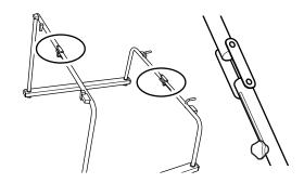
**3-2** Loosen the fixation bolts and slide them into position, then tighten the screws with your hand.
