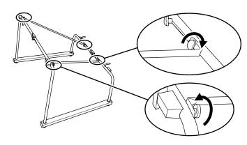
**FNOTE** When removing the braces at disassembly, the screws of the braces may hard to loosen. In this case, loosen the screws while moving the braces lightly to the front, back,
