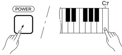
All dual mode, reverb, brilliance (CLP-155), touch sensitivity, and pitch control settings can be restored to their original factory preset values by holding the **C7** key while turning the **[POWER]** switch ON. This also erases all recorder data.
