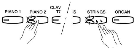
In a DUAL mode voice combination using STRINGS and any other voice, it is possible to switch the STRINGS voice to a slow-attack variation when initially selecting the voices by pressing the [**STRINGS**] selector twice while holding the other voice selector. Repeat this operation to return to the normal STRINGS voice attack.
