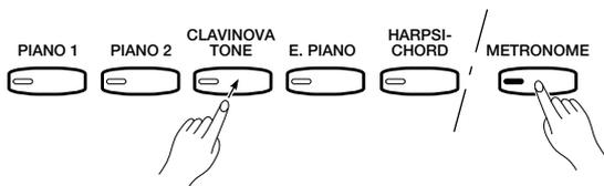
The time signature of the metronome sound can be set by pressing the appropriate voice selector button while holding the [METRONOME] button, as follows:
