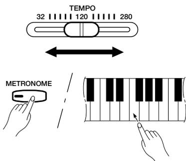
The tempo of the metronome and recorder playback can be controlled in two ways:
