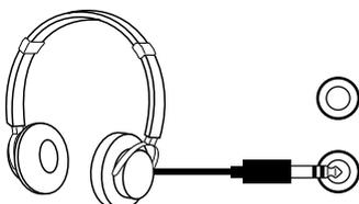
Two pairs of standard pair of stereo headphones can be plugged in here for private practice or late-night playing. The internal speaker system is automatically shut off when a pair of headphones is plugged into either of the PHONES jacks.
