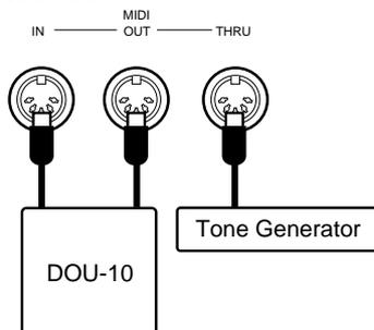
The MIDI IN connector receives MIDI data from an external MIDI device (such as the DOU-10 Disk Orchestra Unit) which can be used to control the Clavinova. The MIDI THRU connector re-transmits any data received at the MIDI IN connector, allowing "chaining" of several MIDI instruments or other devices. The MIDI OUT connector transmits MIDI data generated by the Clavinova (e.g. note and velocity data produced by playing the Clavinova keyboard).
