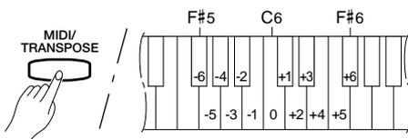
\* Keys **F#5** through **F#6** on the keyboard are used to set the MIDI transmit transpose function as shown in the illustration to the left.
