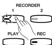
When the record mode is engaged in the previous step, the last-recorded track will automatically be selected for recording and its indicator — i.e. the **[1]** or **[2]** button indicator — will glow red. If you want to record on a different track, press the appropriate track button so that its indicator glows red.
