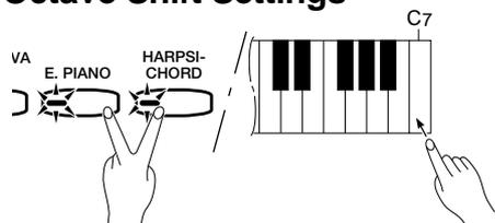
Press the **C7** key while holding any two voice selectors to memorize all balance, STRINGS voice attack variation (CLP-155), and octave shift settings made since the power was turned on. The memorized settings will be retained in memory for about one week after the power is turned off, then the default settings will be restored. To keep the memorized settings for longer periods, turn the power on briefly at least once a week.
