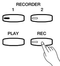
Press either the **RECORDER [REC]** or **[PLAY]** button to stop recording. The indicator of the recorded track will glow green to indicate that it now contains data.
