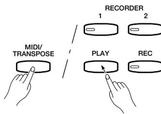
This function is used to transmit all data stored in the Recorder memory to a MIDI data storage device such as the Yamaha DOU-10 Disk Orchestra Unit, other sequence recorders, or MIDI compatible computers.
