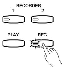
Press the **RECORDER [REC]** button to engage the record ready mode (recording does not actually start yet). The **[REC]** button indicator will light.
