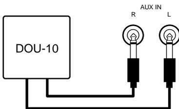
These jacks are intended for use with an external tone generator module such as the Yamaha DOU-10 Disk Orchestra Unit. The stereo outputs from the external tone generator module are connected to the AUX IN L and R jacks, allowing the sound of the tone generator to be reproduced via the Clavinova's internal sound system and speakers.
