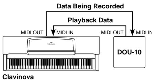
This same type of musical information transfer is used for MIDI sequence recording. A sequence recorder can be used to “record” MIDI data received from a Clavinova, for example. When the recorded data is played back, the Clavinova automatically “plays” the recorded performance in precise detail.
