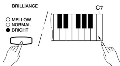
Press the **C7** key while holding the **[BRILLIANCE]** button to memorize the current brilliance setting. The memorized setting will be retained in memory for about one week after the power is turned off, then the default setting (**NORMAL**) will be restored. To keep the memorized setting for longer periods, turn the power on briefly at least once a week.
