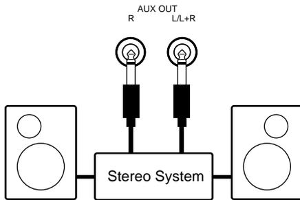
The AUX OUT L/L+R and R jacks deliver the output of the Clavinova for connection to an instrument amplifier, mixing console, PA system, or recording equipment. If you will be connecting the Clavinova to a monaural sound system, use only the L/L+R jack. When a plug is inserted into the L/L+R jack only, the left and right-channel signals are combined and delivered via the L/L+R jack so you don't lose any of the Clavinova's sound.
