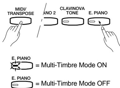
The Multi-Timbre mode is a special mode in which the Clavinova voices can be independently controlled on different MIDI channel numbers by an external MIDI device. The Multi-Timbre mode can be activated as follows:
