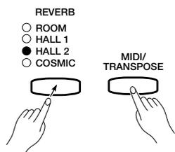
To select a touch sensitivity setting press the [REVERB] button a few times while holding the [MIDI/TRANSPOSE] button until the indicator corresponding to the desired setting lights.
