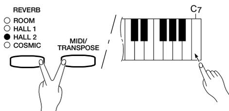
Press the C7 key while holding the [MIDI/TRANSPOSE] and [REVERB] button to memorize the current touch sensitivity setting. The memorized setting will be retained in memory for about one week after the power is turned off, then the default setting (MEDIUM) will be restored. To keep the memorized setting for longer periods, turn the power on briefly at least once a week.
