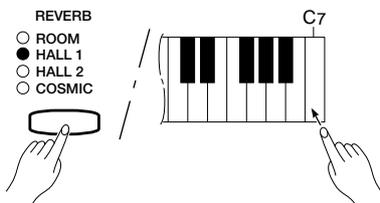
Press the **C7** key while holding the **[REVERB]** button to memorize the current effect type and all depth settings made since the power was turned on. The memorized settings will be retained in memory for about one week after the power is turned off, then the default settings will be restored. To keep the memorized settings for longer periods, turn the power on briefly at least once a week.
