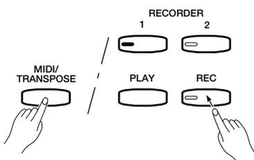
When you want to locate a specific point in a recording you can quickly move forward through the recording while monitoring the sound by pressing the **[REC]** button while holding the **[MIDI/TRANPOSE]** button.
