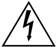
The lightning flash with arrowhead symbol, within the equilateral triangle, is intended to alert the user to the presence of uninsulated "dangerous voltage" within the product's enclosure that may be of sufficient magnitude to constitute a risk of electrical shock.
