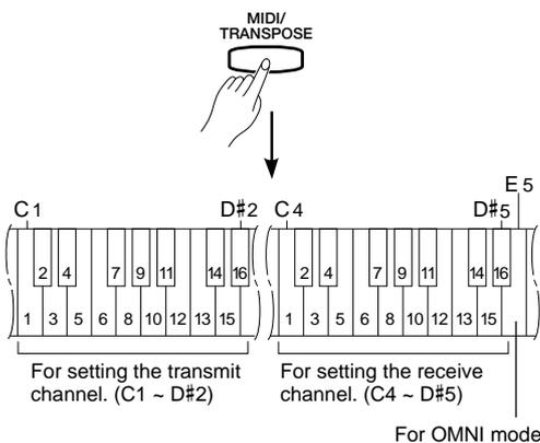
\* Keys **C1** through **D#2** on the keyboard are used to set the MIDI transmit channel, and keys **C4** through **D#5** are used to turn the OMNI mode OFF and set the MIDI receive channel as shown in the illustration to the left. The **E5** key sets the OMNI receive mode and basic receive channel 1.
