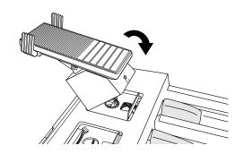
Fix the expression pedal to the pedal unit while holding the expression pedal, using the screw you removed in step 2-2.
