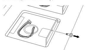
4-3 Hold the cable connector so that the two lines on the connector are facing upward, then carefully plug it into the inside connector on the bottom of the second expression pedal.
