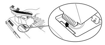
Fix the 2nd expression pedal to the pedal unit while holding the 2nd expression pedal, using the screw you removed in step 4-2.
