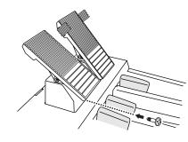
Connect the TO MAIN terminal of the Pedalboard to the TO PEDAL terminal of the instrument using the cord.
