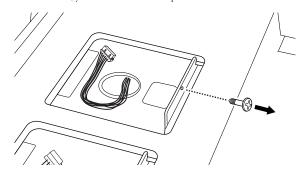
**2-3** Hold the cable connector so that the two lines on the connector are facing upward, then carefully plug it into the inside connector on the bottom of the expression pedal.
