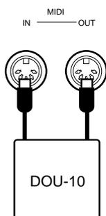
The MIDI IN connector receives MIDI data from an external MIDI device (such as the DOU-10 Disk Orchestra Unit) which can be used to control the Clavinova. The MIDI OUT connector transmits MIDI data generated by the Clavinova (e.g. note and velocity data produced by playing the Clavinova keyboard).
