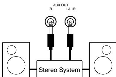
The AUX OUT R and L/L+R jacks deliver the output of the Clavinova for connection to an instrument amplifier, mixing console, PA system, or recording equipment. If you will be connecting the Clavinova to a monaural sound system, use only the L/L+R jack. When a plug is inserted into the L/L+R jack only, the left- and right-channel signals are combined and delivered via the L/L+R jack so you don't lose any of the Clavinova's sound.
