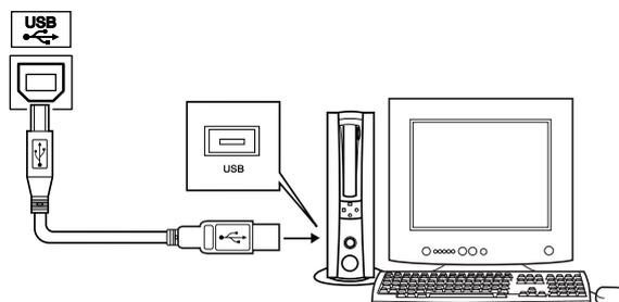
Connect the instrument's USB terminal to the USB terminal of a computer, and you can transfer performance data and song files between the two (page 79). To use the USB data-transfer features you'll need to do the following:
