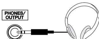
The DGX-230/YPG-235 speakers are automatically shut off when a plug is inserted into this jack.
