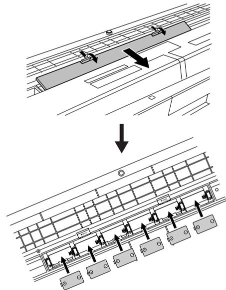
For battery operation the instrument requires six 1.5V "D" size, R20P (LR20) or equivalent batteries. (Alkaline batteries are recommended.) When battery power becomes too low for proper operation, make sure to replace all batteries, following the precautions listed below.
