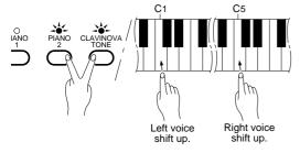
Depending on which voices you combine using the DUAL mode, the combination may sound better if one of the voices is shifted up an octave. To shift the right voice, press the C5 key while pressing the two voice selectors corresponding to the voices to be combined in the DUAL mode. Press C5 again to shift the voice back to its normal range. Use the C1 key in the same way to shift the left voice.
