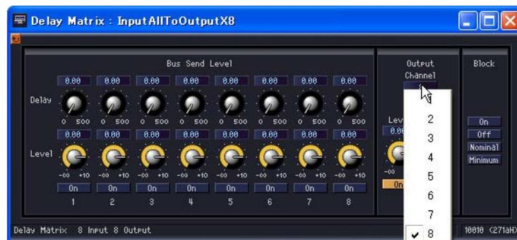
If you make the delay matrix component editor active while the [Delay Matrix - All Inputs to One Output] editor window is displayed, and then click another output channel, that channel group will be displayed in the [Delay Matrix - All Inputs to One Output] editor window. One [Delay Matrix - All Inputs to One Output] editor window is displayed for each delay matrix component editor.
