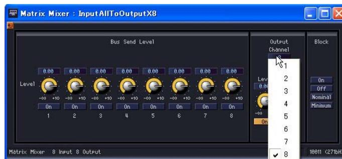
If you make the matrix mixer component editor active while the [Matrix Mixer - All Inputs to One Output] editor window is displayed, and then click another output channel, that channel group will be displayed in the [Matrix Mixer - All Inputs to One Output] editor window. One [Matrix Mixer - All Inputs to One Output] editor window is displayed for each matrix mixer component editor.
