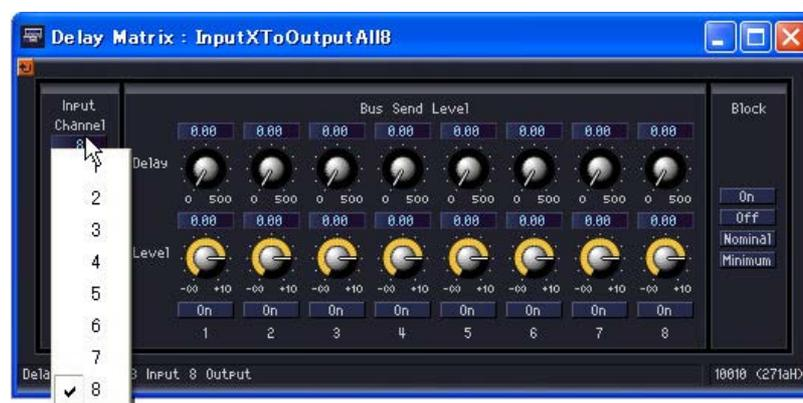
If you make the delay matrix component editor active while the [Delay Matrix - One Input to All Outputs] editor window is displayed, and then click another input channel, that channel will be displayed in the [Delay Matrix - One Input to All Outputs] editor window. One [Delay Matrix - One Input to All Outputs] editor window is displayed for each delay matrix component editor.
