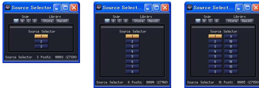
The Source Selector connects the selected input to the output. For example, if you select [1] for a 4 Position 2 Channel component, IN1-1 will be connected to OUT-1 and IN1-2 will be connected to OUT2. If you select [2] IN2-1 will be connected to OUT-1 and IN2-2 will be connected to OUT2.
