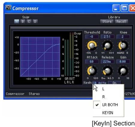
The currently selected trigger source is displayed on the button. Click the button and select the trigger source from the menu.
