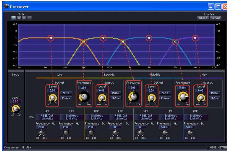
You can adjust the [Output Level] parameter by vertically dragging the control point in the center of each curve.
