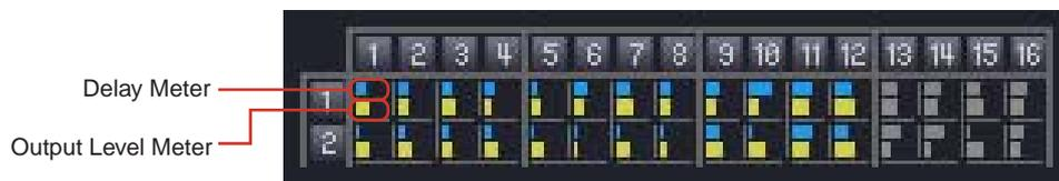
When you click the output channel number on the matrix, the [Delay Matrix - All Inputs to One Output] editor window opens. When you click the input channel number on the left side of the matrix, the [Delay Matrix - One Input to All Outputs] editor window opens.
