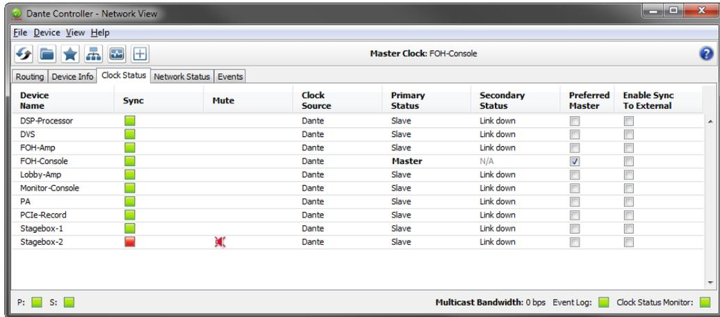
Figure 6: Dante Controller "Clock Status" tab
