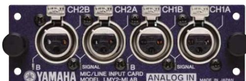
2-channel analog input card equipped with A/B select switch compatible with mic/line level. Each channel is independent and A/B input switching, gain trimming (-68dB ~ +10dB) and phantom power supply on/off can be controlled from CS1D. With the newly developed built-in head amplifier, richer and fuller sound quality is realized. 28-bit equivalent high-quality sound with dynamic range exceeding 120dB is realized by the AD floating control. Up to 8 cards can be mounted to A18.
