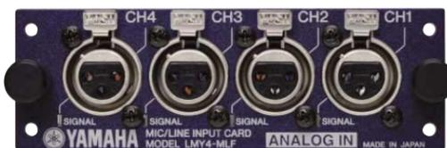
4-channel analog input card compatible with mic/line level. Gain trimming (-68dB ~ +10dB) and phantom power supply on/off of each channel can be controlled from CS1D. With the newly developed built-in head amplifier, richer and fuller high-quality sound is realized with dynamic range exceeding 110dB. Up to 8 cards can be mounted to A18.
