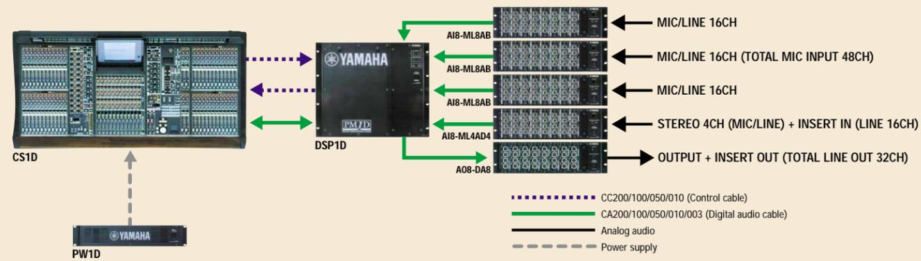
Basic 48-channel system. Three AI8-ML8AB mic/line input units are used for mic/line input of 48 channels in total. Using mic/line/AD unit AI8-ML4AD4, 4 stereo inputs and 16 line inputs for insert-in are provided. Including insert-out, a total of 32 outputs are provided by the DA unit AO8-DA8.
