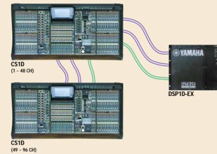
System that controls input of 96 channels + 8ST from DSP1D-EX without using layers. By using two CS1D units, all input are expanded to the fader to realize speedy control and superior visibility of all input levels of 96 channels + 8ST and panning displayed as lists. For fail-safe operation, 2 CONSOLE IN/OUT terminals are also provided.
