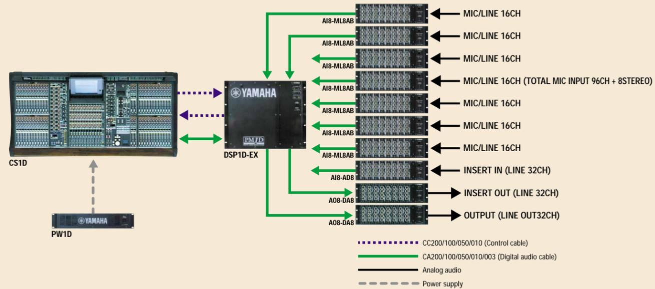
The 96-channel system uses seven AI8-ML8AB mic/line input units for input. Mic/line input of 112 channels is available and one of the units is input to 8 stereo inputs. AD unit AI8-AD8 is used for insert-in, providing line input of 32 channels in total. Furthermore, DA unit AO8-DA8 is used for insert-out, providing line output of 32 channels in total. AO8-DA8 is also used for output, providing output of 32 channels in total.
