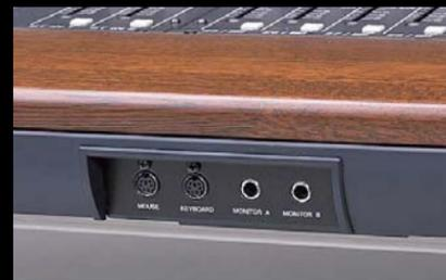
The front panel is equipped with mouse and keyboard terminals.
