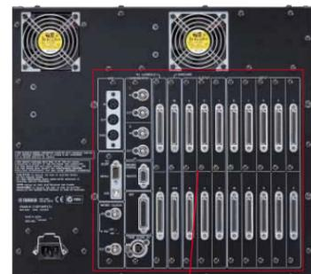
DSP1D (-EX) is equipped with a power supply cable lock on the power supply connector section to prevent problems such as disconnection of the power cable, etc.
