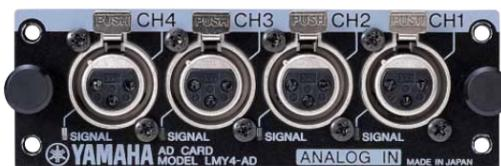
4-channel analog input card compatible with line level. 28-bit equivalent high-quality sound with dynamic range exceeding 120dB is realized by the AD floating control. Up to 8 cards can be mounted to A18.
